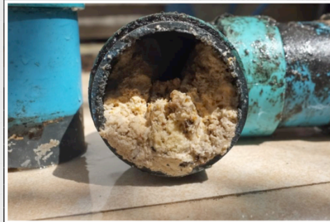
Pipe clogged with fats and grease
